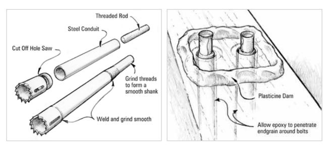
**Figure 4-13** A custom keel bolt saw can be made from a pipe section and a standard hole saw.
