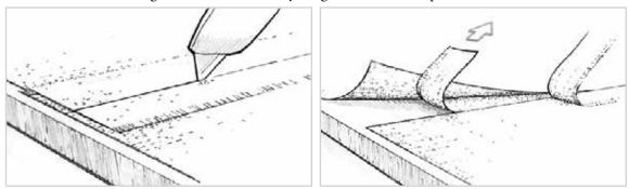
Figure 8-20 Trim overlapping fabric using a metal straightedge Figure 8-21 Remove the topmost trimming. Then lift the and a sharp utility knife, for a flush butt joint.
