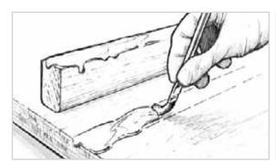
**Figure 8-8** Wet out bonding surfaces with unthickened epoxy for maximum penetration and greater adhesion.
