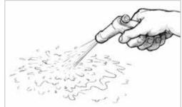
Figure 7-6 *Rinse water should sheet without beading, indicating an uncontaminated surface.*
