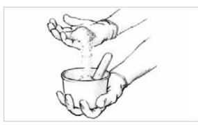
**Figure 8-7** Blend in small handfuls or scoops of the appropriate filler until the desired consistency is reached.
