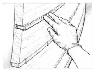
Figure 5-4 Push the wet-out spline into the seam.
