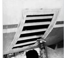
**Figure 5-16** *Bevel the edges and fasten temporary stringers to the back of the opening.*
