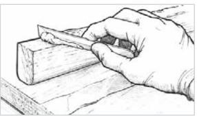
**Figure 8-9** Apply enough thickened epoxy to one of the bonding surfaces so that a small amount will squeeze out of the joint when clamped with moderate pressure.
