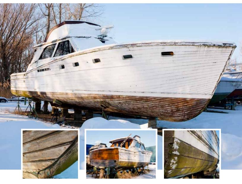
A guide to restore the structure, improve the appearance, reduce the maintenance and prolong the life of wooden boats with WEST SYSTEM<sup>®</sup> Epoxy.
