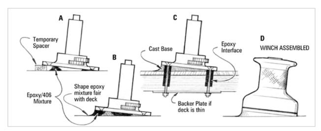
Figure 6-3 Hardware casting is an excellent method for installing a piece of hardware that is not flush to the deck such as a winch.
