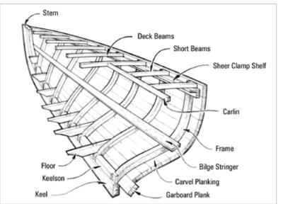
Figure 2-1 Typical structural framework.
