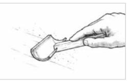
**Figure 7-4** *Tip off the coating by dragging a foam roller brush lightly over the fresh epoxy.*
