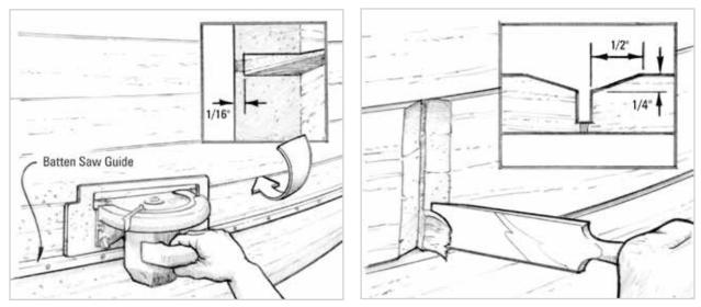
**Figure 5-1** Use a circular saw to clean out plank seams.
