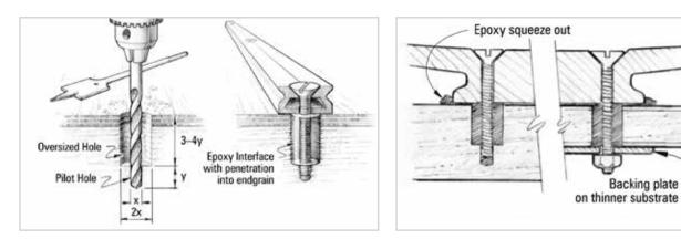
**Figure 6-1** A normal sized pilot hole at the bottom of the oversized hole provides enough clamping pressure to hold the hardware in position until the epoxy cures.
