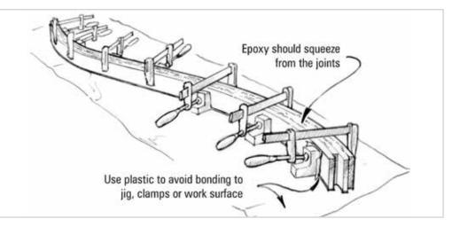
Figure 4-2 Clamp the appropriate number of coated strips into the jig. Trim the frame to size after the epoxy is fully cured.
