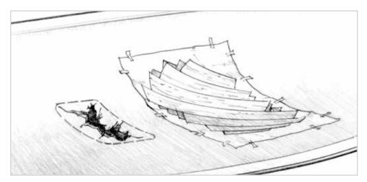
Figure 5-20 Laminate a replacement panel using the surface next to the damaged area as a mold.
