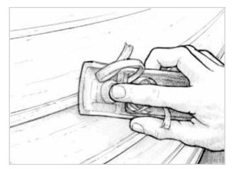
**Figure 5-5** Use a plane to remove the excess spline and a sander to fair the surface after the epoxy has cured.
