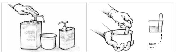
**Figure 8-4** *Dispense the proper proportions of resin and hardener.*
