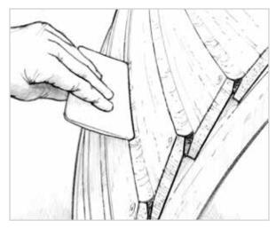
Figure 5-8 Clean out the seams with a scraper.
