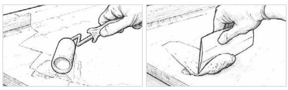
**Figure 8-14** Wet out porous surfaces before applying thickened fairing compound.
