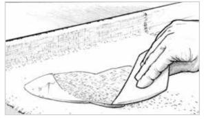
**Figure 8-17** *Spread the epoxy from the center of the fabric toward the edges with a plastic spreader.*
