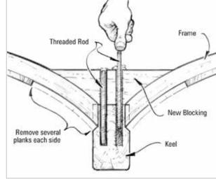
Figure 4-10 Bond new floors and blocking to the keels and frames.
