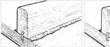
**Figure 8-10** A small amount of epoxy will squeeze out of the joint with just the right amount of thickened mixture and clamping pressure.
