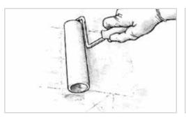
**Figure 7-3** *Roll lightly and randomly over a small area. Spread the epoxy into a thin even film.*
