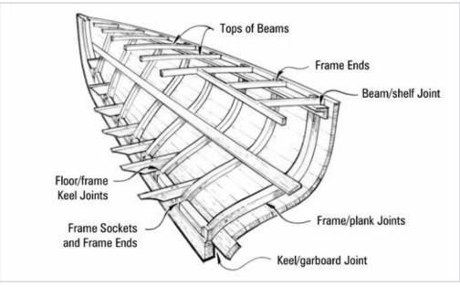
Figure 2-4 Look for dry rot at joints and areas of standing water and poor air circulation
