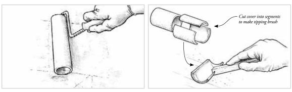
**Figure 8-23** Apply the epoxy in thin even coats using a thin foam roller.
