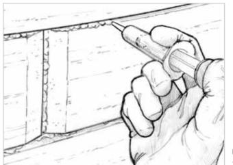
**Figure 5-3** Inject G/flex 655 into the wet-out seam.
