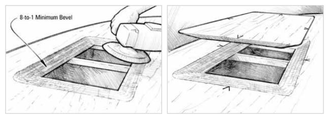
**Figure 5-12** *Cut out the damaged area and grind a minimum 8-to-I bevel on all sides of the opening.*
