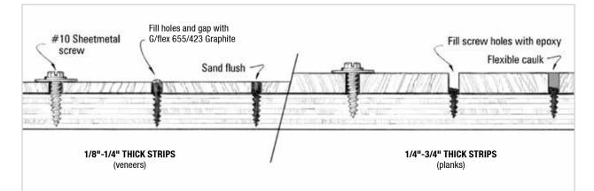
Figure 5-24 Sheet metal screws with large washers will clamp the strips in position until the 655/graphite mixture cures thoroughly.
