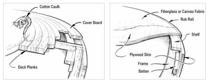
Figure 2-2 Typical laid plank deck and carvel planked hull.
