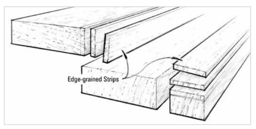
Figure 5-23 Thin edge-grained strips provide an even wearing, attractive and dimensionally stable deck.
