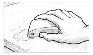
**Figure 8-16** *Sand the fairing material to blend with the surrounding contour.*
