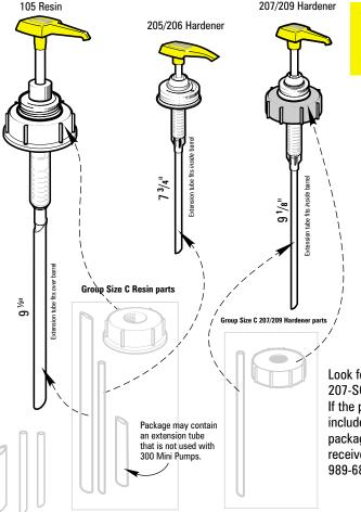
WARNING! 300 Mini Pumps have yellow heads. Do not use a 300 Mini Pump in combination with any pump with a white head.
