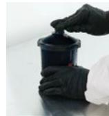
**7** Use the 3M™ PPS™ Series 2.0 Cup Sealing Plug to seal and protect coatings not in use, in accordance with local regulations or authorities. Be sure to see Pro Tips section for easy lid and liner removal from hard cup.
