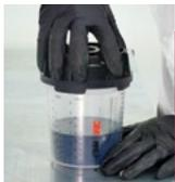
**4** Optional: Insert cup sealing plug into lid spout. Use the 3M™ PPS™ Series 2.0 Universal Shaker Core on top of any size cup and place into paint shaker. When paint is mixed, remove shaker core and sealing plug.
