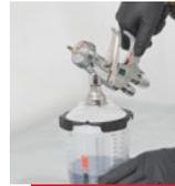
**5** Choose the right adapter for your spray gun. Push down and twist until adapter locks into lid. (Go to [3MCollision.com/PPSadapters](http://3MCollision.com/PPSadapters) to find the adapter that fits your spray gun.)
