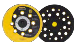
915GV28 * 5" Backup Pad Medium, Multi-Hole, Grip 5/16" - 24 thread
