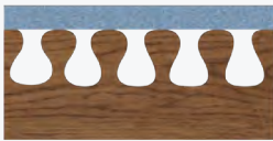
Finish sits on top of the surface leading to cracking, peeling, blistering and flaking
