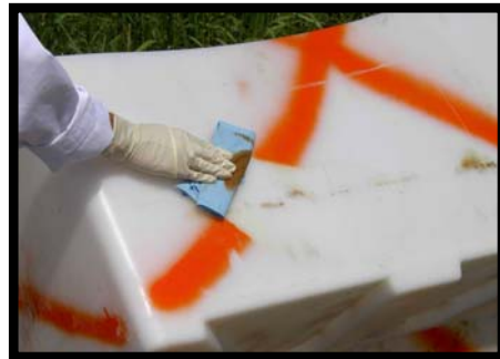
Removing spray paint from a plastic Media (polyethylene)
