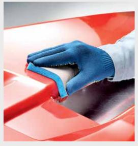
**Manual sanding of hard-to-reach areas** e.g. keying/sanding of plastic parts, intermediate sanding in hard-to-reach areas
