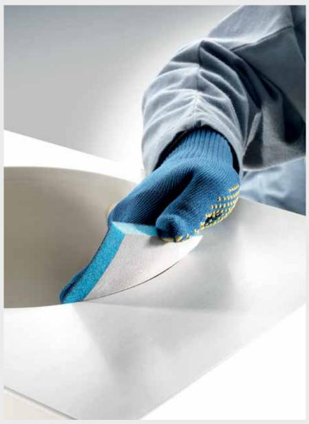
**Manual sanding of contours and edges** e.g. preparation for painting over painted workpieces
