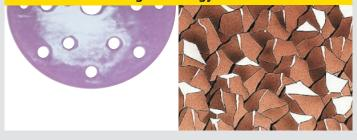
The original technology uses closed coating according to an electrostatic process. The "New Generation" technology improves the positioning of the abrasive grains with open coating. This results in over 20% better removal rate with minimal clogging.
